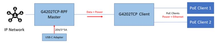
Variant 2: G4202TCP as client together with G4201C Master. G4202TCP draws power from the USB-C adapter.
