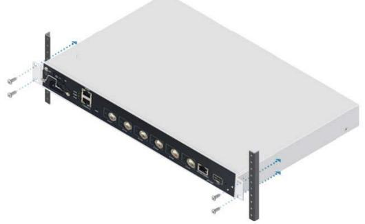
c) If there is no screw hole on the rack rail and the holes on the rack rail are square, first insert the cage nuts to the proper holes on the rail from the far side, then install the rack-mount screws through the holes of the mounting bracket onto the cage nuts to mount G4200C to the rack, two mounting screws on each side.
