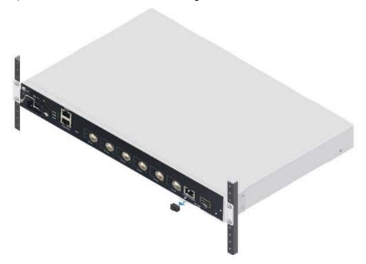
b) Insert SFP transceiver into the SFP cage
