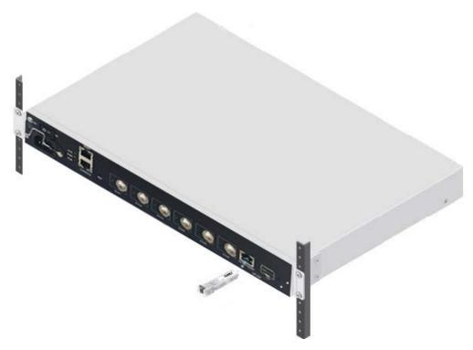
c) Connect optical fiber to the SFP transceiver and coaxial cable to the G.hn port(s) respectively
