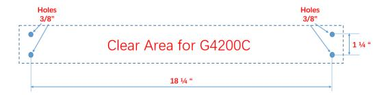
c) Nail in four wall-mount plastic nuts into four drill holes, then mount G4200C on the wall with four wall-mount screws.
