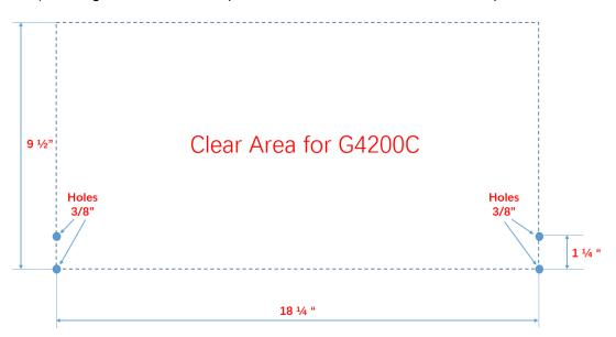
c) Nail in four wall-mount plastic nuts into four drill holes, then mount G4200C on the wall with four wall-mount screws.
